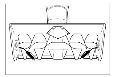
Figure 4. Auger Bearing Lubrication
